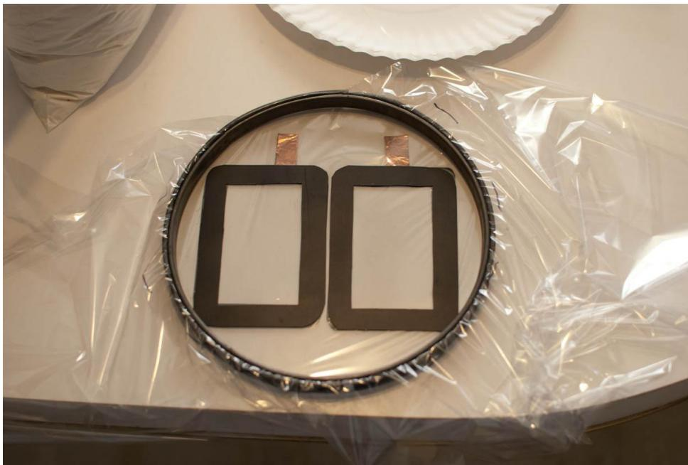
After the Insulator rings were set, the perforated panels were cut to the same size and glued to the outside of the insulator rings. The edges of the Mylar were then cut, and all edges were covered with electrical tape.
