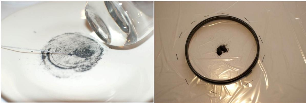
In the finished product, it can be noted that the graphite impregnated Mylar is darker than the untreated:
