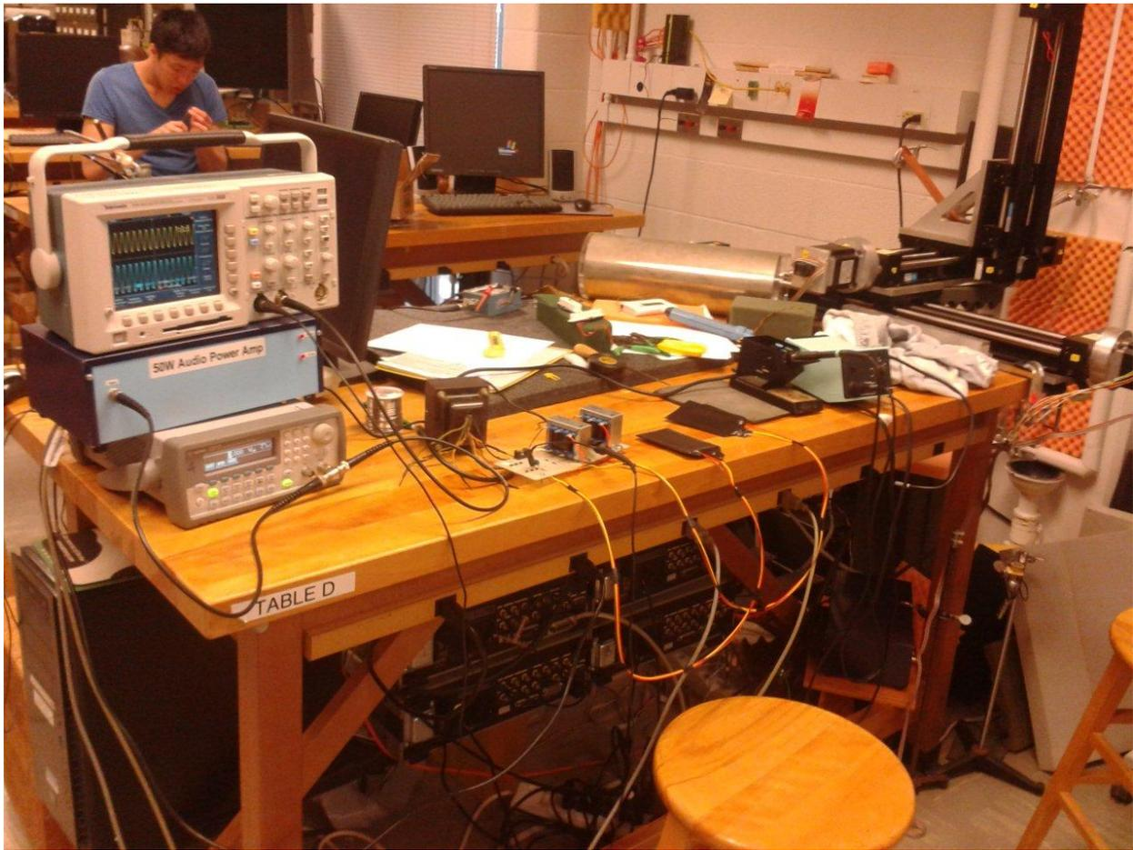
The blue signal on the oscilloscope is the reference signal from the sine wave generator and the yellow is the voltage output from the Edcor audio transformers. Both channels produced audible sound with this setup.
