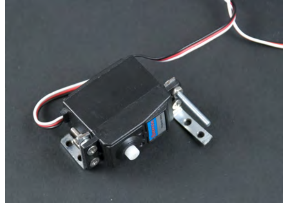
Figure 8-33. Kicker servo attachments from above
