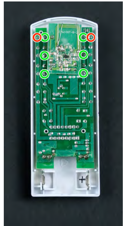
Figure 7-13. Solder pads: red wires to red ones and green wires to green ones
