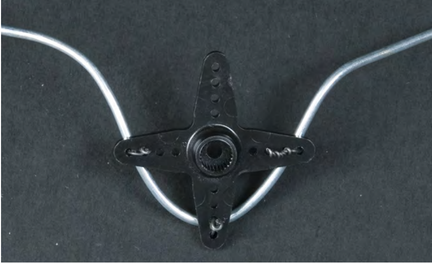
Figure 4-10. Attaching with metal wire
