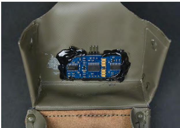
Figure 3-28. A hot-glued ultrasonic sensor
