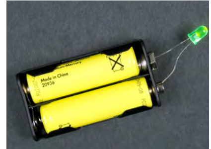
Figure 1-28. Simple closed circuit powering an LED
