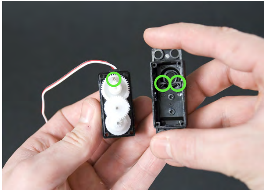
Figure 8-9. Obstructions that block rotation
