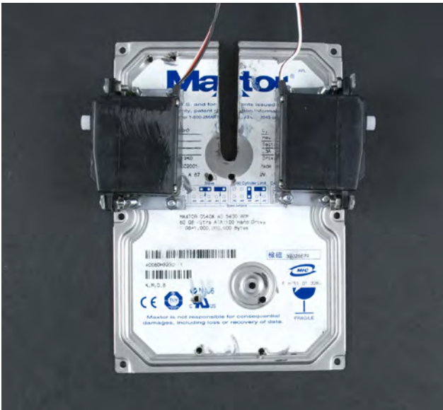
Figure 8-38. Attached wheel servos from below
