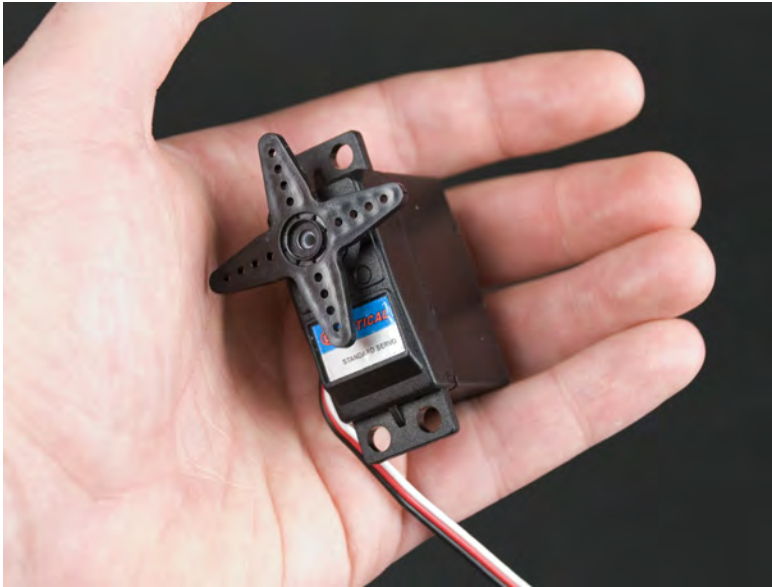
Figure 8-17. Finished continuous rotation servo
