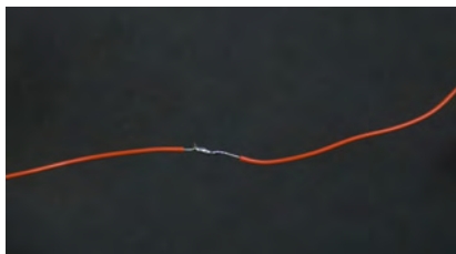
Figure 3-38. Finished soldered joint
