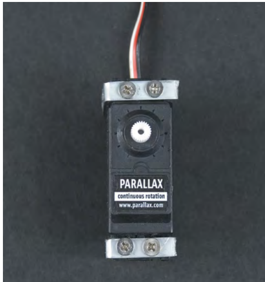
Figure 8-34. Wheel servo attachments from the front
