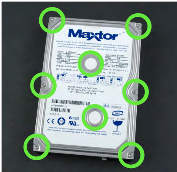
Figure 8-26. Locations of screws
