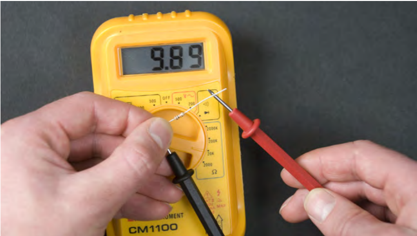
Figure 5-6. Measuring resistance with a multimeter
