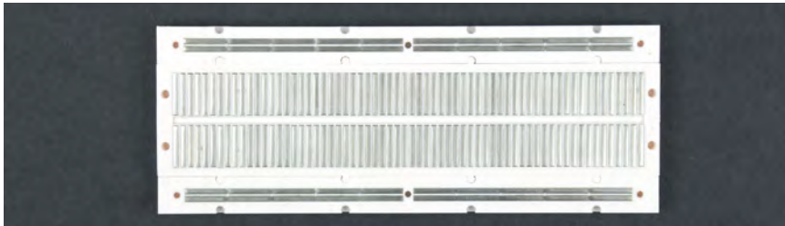
Figure 3-5. View of the bottom of the prototyping breadboard; metal plates conduct current from hole to hole
