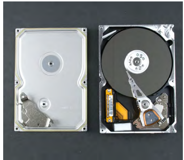
Figure 8-27. Hard drive opened
