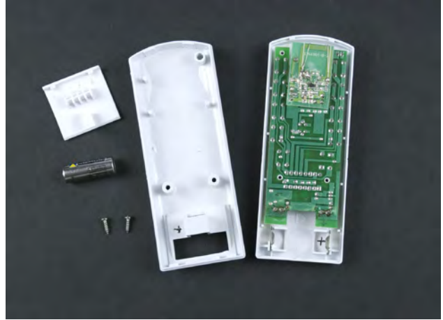
Figure 7-10. Opened remote control
