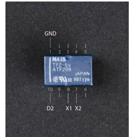
Figure 7-4. Relay circuit connections
