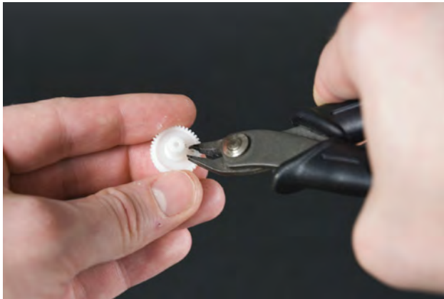
Figure 8-10. Cutting off the obstructions
