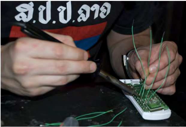
Figure 7-15. Soldering wires to the remote control switches
