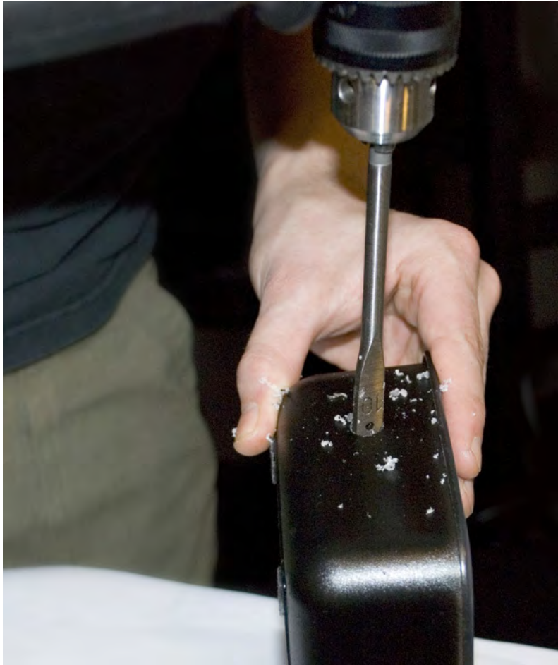
Figure 7-33. Drilling a hole for the USB cable
