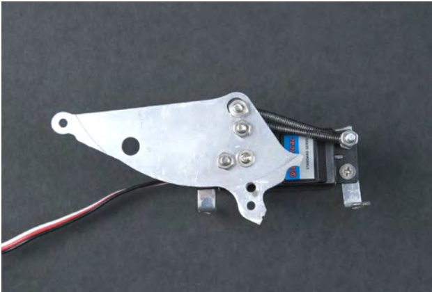
Figure 8-46. Kicker leg attached to the servo
