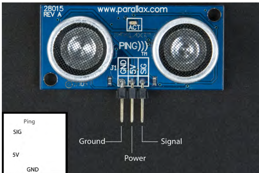
Figure 3-8. The Ping))) ultrasonic sensor
