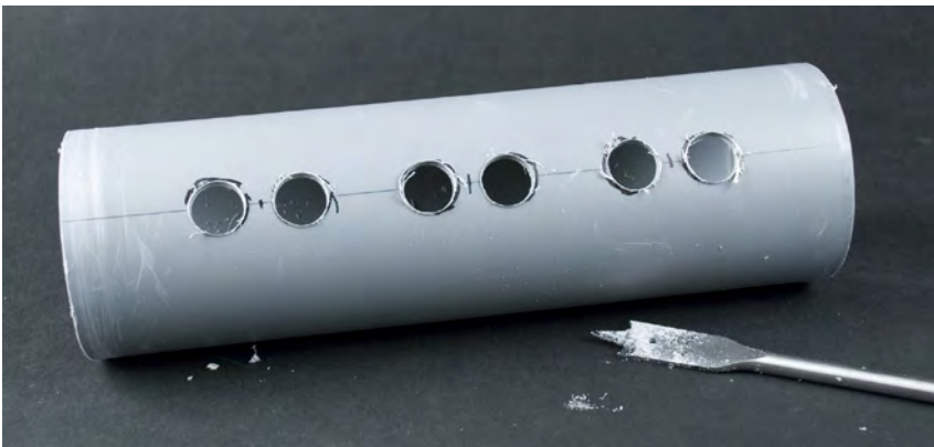
Figure 5-29. The 16mm holes for the sensors
