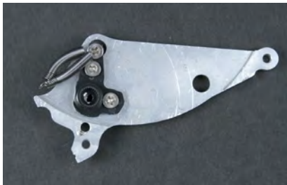
Figure 8-45. Kicker leg with servo horn attached
