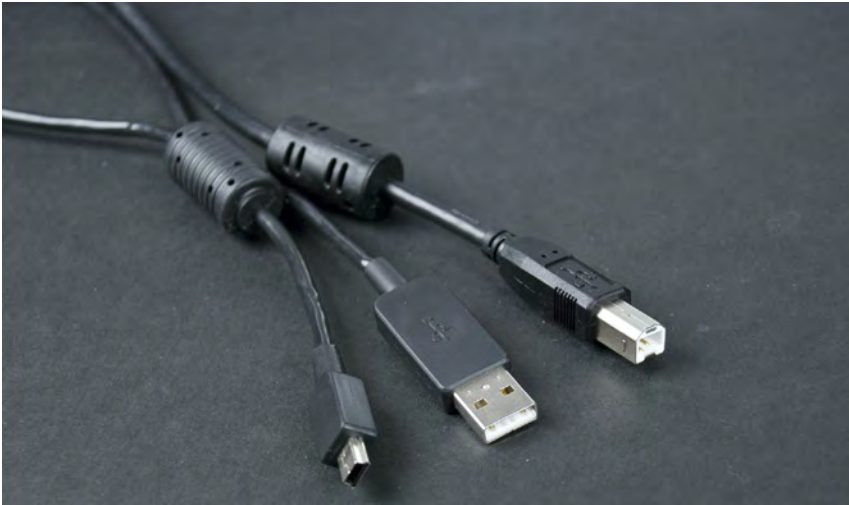
Figure 2-3. Arduino USB cables: Mini-B, USB-A, and USB-B
