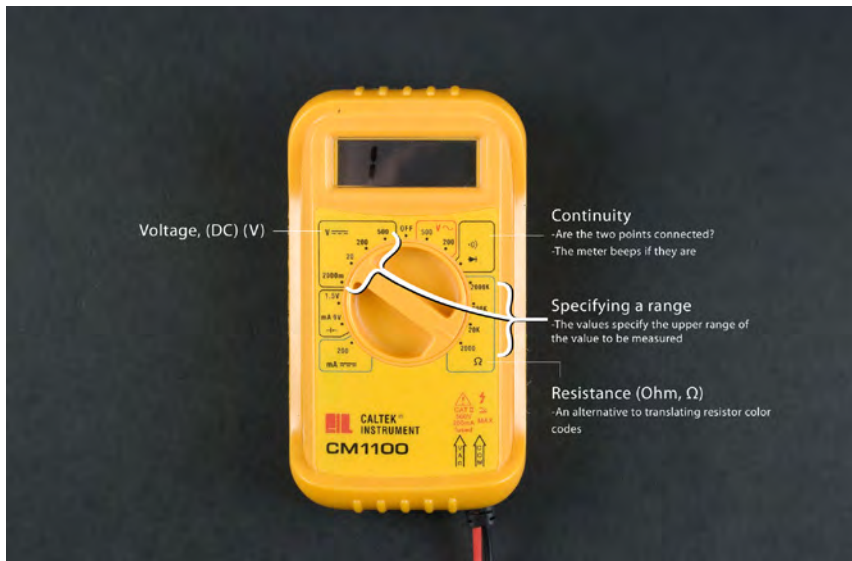
Figure 1-26. The most common functions of a multimeter
