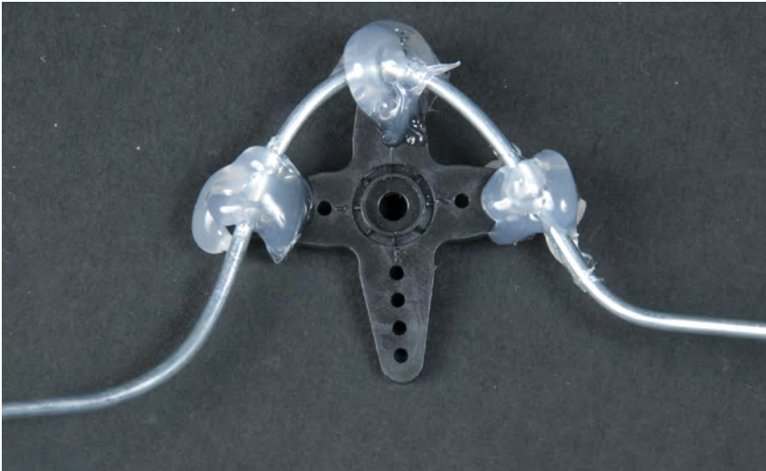
Figure 4-11. Securing with hot glue
