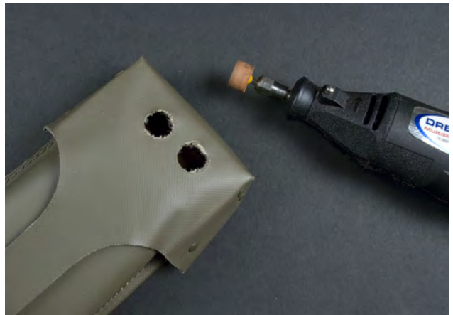
Figure 3-27. Holes created with a mini drill
