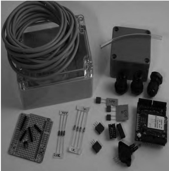
Figure 12-1. Parts required for water tank depth sensor
