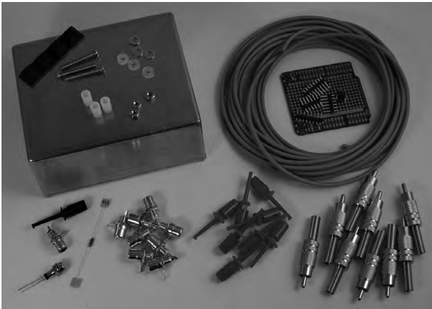
Figure 11-2. Parts required for Arduino Oscilloscope / Logic Analyzer
