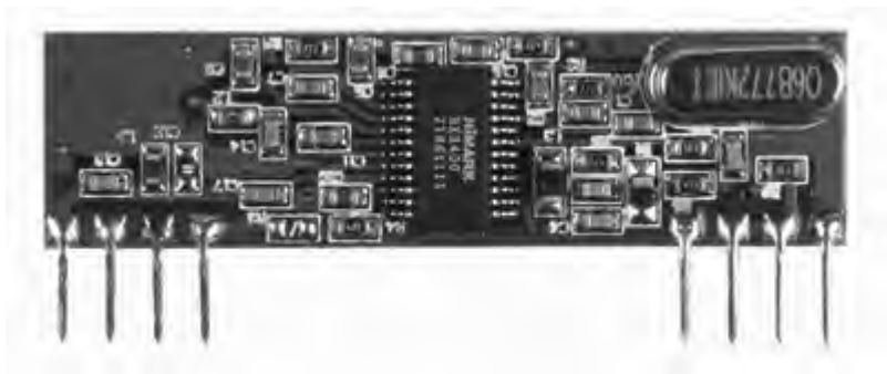
Figure 13-5. RXB1 433MHz receiver module
