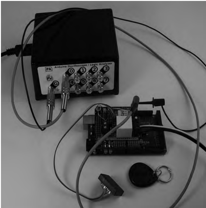
Figure 11-10. Connection to a circuit under test
