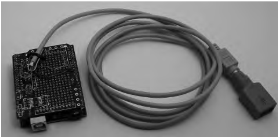
Figure 5-9. PS/2 extension cable attached to shield
